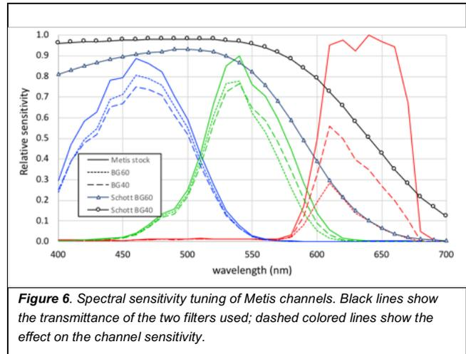
Figure 6. Spectral sensitivity tuning of Metis channels. Black lines show the transmittance of the two filters used; dashed colored lines show the effect on the channel sensitivity.
