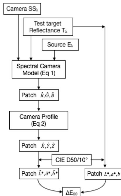
**Figure 3b.** Complete spectral workflow showing the use of the spectral sensitivities and target spectral reflectance for the prediction of  $\hat{R}, \hat{G}, \hat{B}$  camera output. The forward profile predicts tristimulus values, which after conversion to CIELAB are compared to the measured target color.
