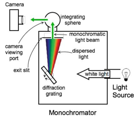
**Figure 1.** Experimental apparatus to present near monochromatic stimuli to camera system. The diffraction grating is rotated, changing the wavelength of light incident on the exit slit. In this fashion the entire visible spectrum can be imaged in sequence, one wavelength band at a time.
